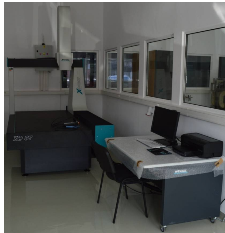
XOrbit 87-1500 Next Generation Coordinate Measuring Machine from WENZEL Prazision GmbH
